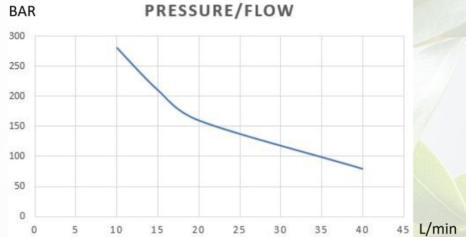
**Variable Piston Pump: A10VS028 DFLR/31R**
