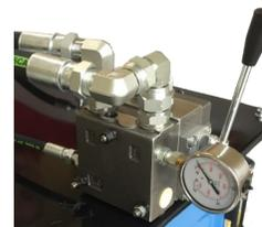
**Hydraulic valve: Standard PV-140, 1 section.**
