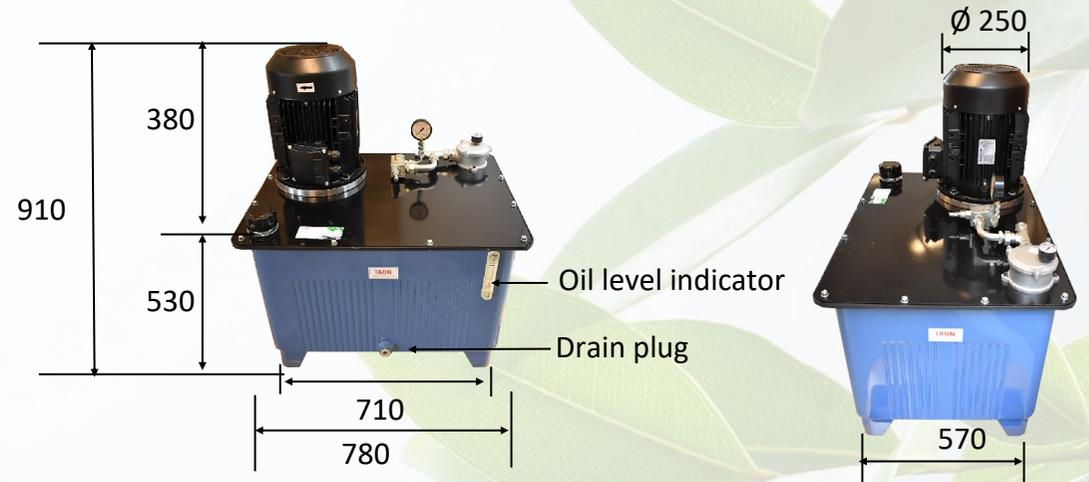
This Hydraulic Power Unit comes with a double pump at 8+22 cm<sup>3</sup> with high/low function.
