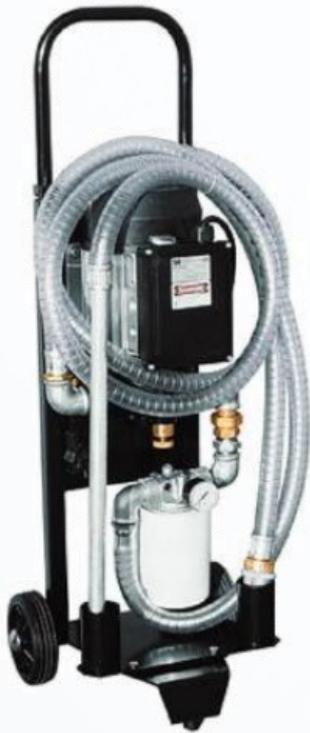
The hydraulic filtration system removes solid contamination and water from petroleum based fluids such as hydraulic fluid and gear and lube oils. The filter cart can be used to pre-filter fluids, transfer fluids or to clean existing systems.
